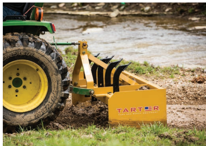
Ripper shanks can be raised completely for bucket-only operation.
