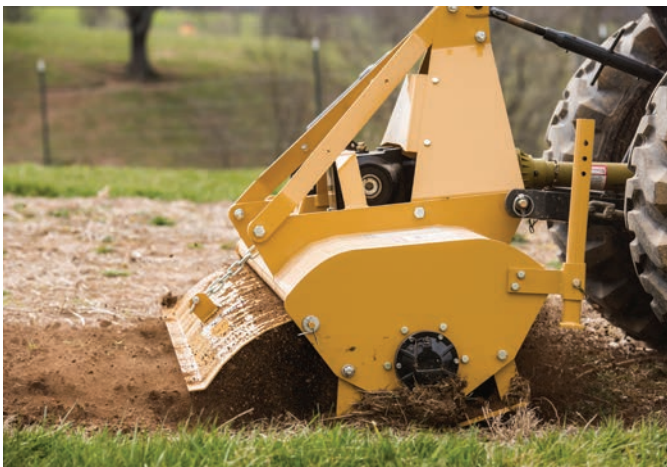
Heavy duty tines provide a digging depth of up to 7".
