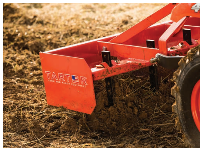
Ripper shanks help break up hard or compacted ground.
