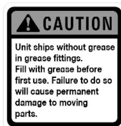
⑤ GREASE CAUTION
