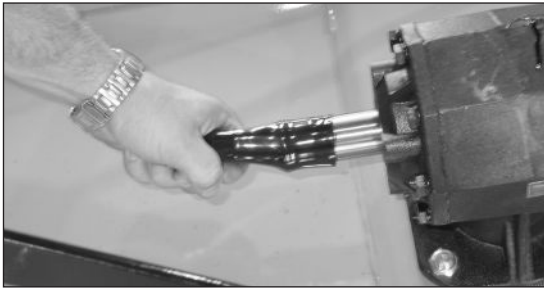
9. Remove shaft boot on PTO gearbox.
