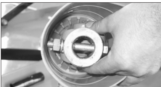
12. Remove PTO shear bolt from end of shaft.
